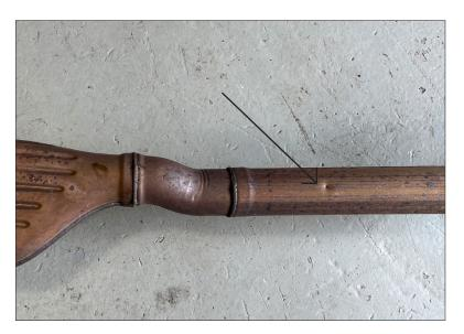
Remove entire Cat-back system from the car, MINI put a dimple in the pipe which is the factory cut point, we have used the same point for our system. Make a cut on the dimple shown in the photos.
